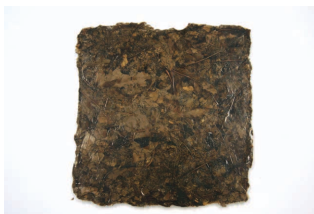
Figure 5. Composite panel prepared using VARTM with AESO and northern red oak ( Quercus robur ) leaves treated with B–E– \gamma -MPS. [Color figure can be viewed in the online issue, which is available at wileyonlinelibrary.com .]
